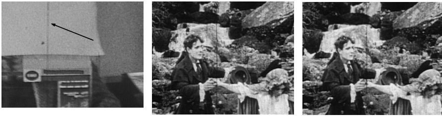
Figure 7.10 Line scratches manifest in much archived footage. They also occur due to accidents in film developing. The color of the scratch depends on which side of the film layer it occurs. Often, not all the image information inside the scratch is lost. Line scratches are a challenge to remove because they persist in the same location from frame to frame.
