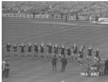
Figure 7.5 Kinescope moiré is caused by aliasing during Telecine conversion and manifests as rings of degradation that move slightly from frame to frame.
