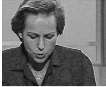
Figure 7.8 Echoes and overshoots manifest as image shadows slightly displaced from each object in the frame. When the effect is severe, it is called echo. When it is limited to just the edges, as in this case, it is called overshoot.
