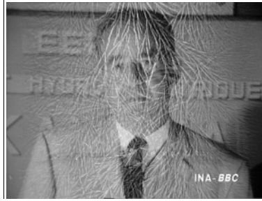
Figure 7.7 Vinegar syndrome often results in a catastrophic breakdown of the film emulsion. This example shows long strands of missing data over the frame.
