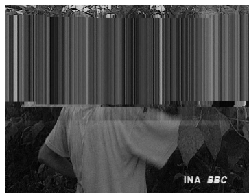
Figure 7.3 Betacam dropout manifests due to errors on Betacam tape. It is a missing data effect in which several field lines are repeated for a portion of the frame. The repeating field lines are the machine's mechanism for interpolating the missing data.
