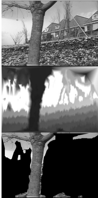
Figure 2.15 Results for the “Flowergarden” sequence using the G8PSFM method. (Source: From R.S. Jasinschi, T. Naveen, A.J. Tabatabai, and P. Babic-Vovk, IEEE Transactions on Circuits and Systems for Video Technology, 10(7): October 2000.)
