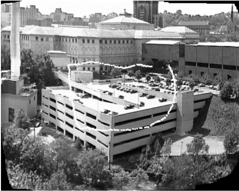
Figure 2.10 The background mosaic for the “Oakland” sequence. It also shows the trajectory of the camera center as it moves to capture the 300 frames. (Source: From R.S. Jasinschi, J.M.F. Moura, J.C. Cheng, and A. Asif, Proceedings of IEEE ICASSP, 1995.)
