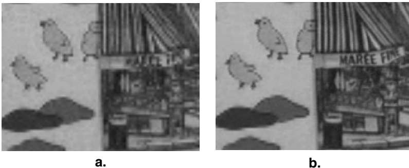
Figure 9.10 (a) Bilinear interpolation of an LR compressed image; (b) image obtained when the whole HR sequence is processed simultaneously.
